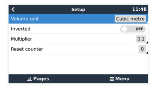
For other sensors and alarms, you can decide whether the input should be treated as an alarm condition, whether the labels should be inverted, and whether the logical levels should be inverted.
