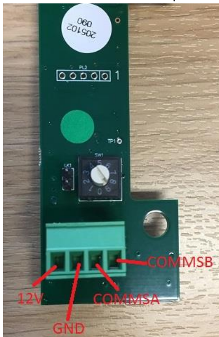
Figure 5 - Wiring connection for the eoMini
