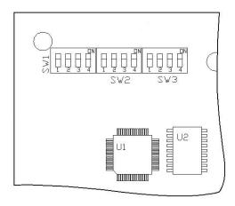
**SW1** dip-switch 2, 3, 4 set the maximum current of the charger. See table below for the dip-switches settings
