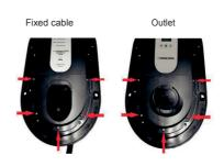
6. Use 4 wood screws M4,5x35mm to mount Charging Station on the wall. The Charging Station should be installed between 0,80m and 1,20m from bottom to the ground.
