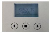
Hold the center button for 2 seconds to enter the menu. You can now use the left and right buttons to go to the different menu options.
