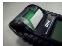
C. Place a small length of paper from the compartment and press the transparent cover to close.
