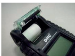
B. Place a new roll of paper in the compartment. Reference paper : 056237 or 056633
