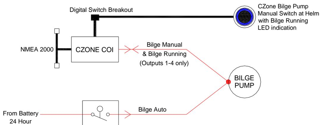
Figure 9. COI Bilge Pump Wiring Example
