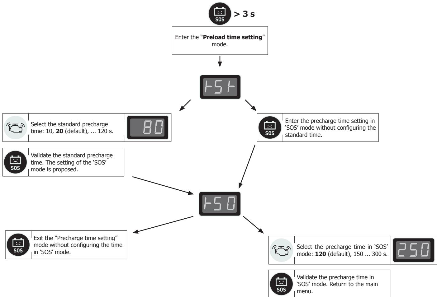
**! In SOS mode, there are no more protections (on the 12 V / 24 V voltage, in case of polarity reversal...). The time setting can damage the battery:**
