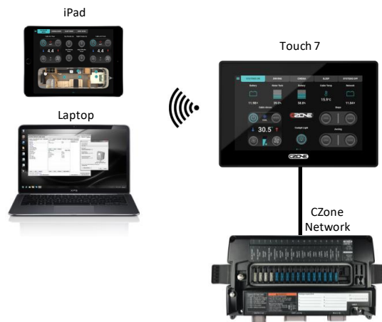
Figure 4. Access Point Example
