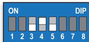
#3 OFF / #4 ON / #5 OFF DEEP CYCLE LEAD ACID
