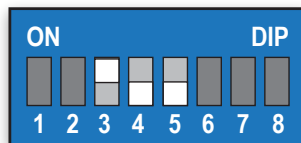
#3 ON / #4 OFF / #5 OFF STANDARD LEAD ACID
