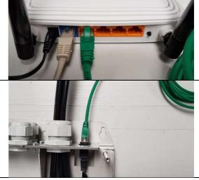
The Router is preconfigured there is no additional configuration or setup necessary. As soon as the router is connected to the internet and the combiner box is turned on the combiner box will automatically establish a connection to our server.
