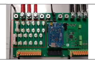
After inserting the fuses, the Combiner Box is ready to go. The Inverters can now be powered up. The system should start-up and will continue operation.
