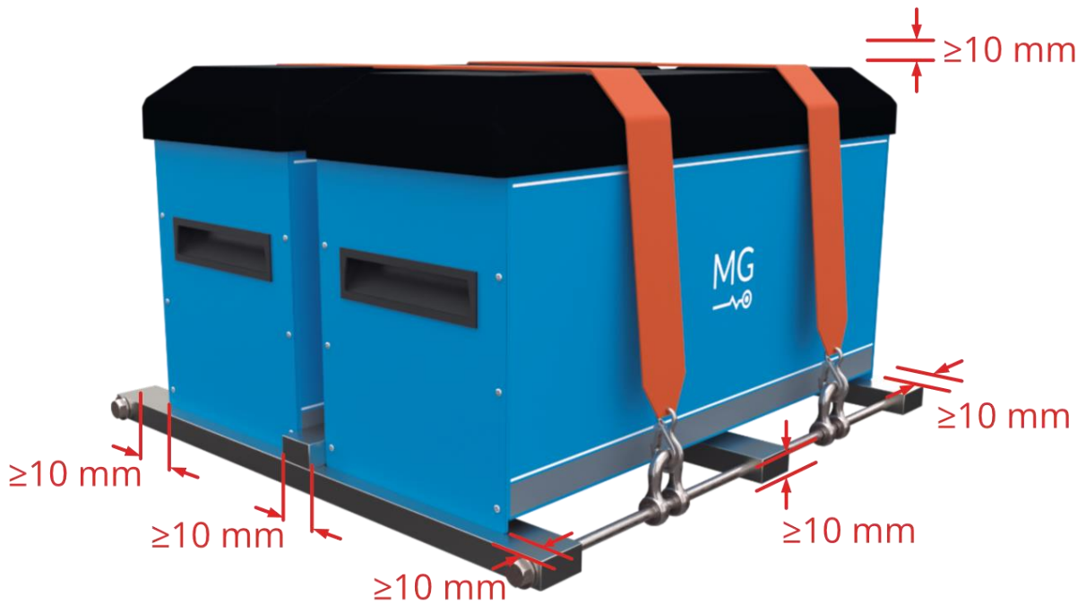
Figure 12 - Battery spacing requirements
